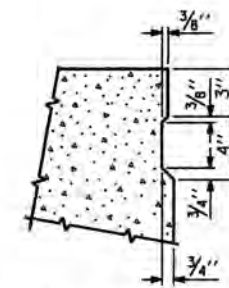
SHEAR KEY DETAIL
